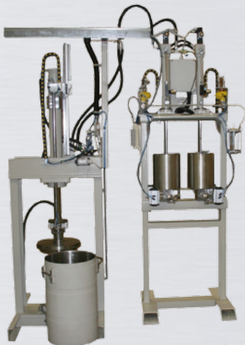
Detail: vessel press for catalyst with double buffer vacuum system
